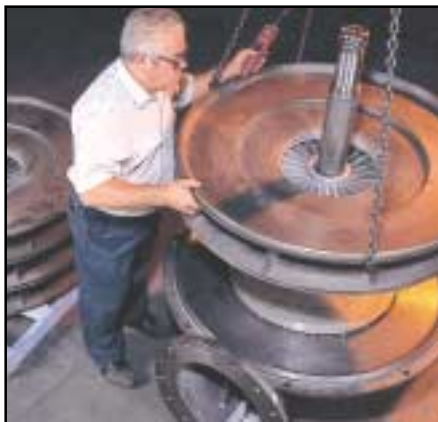
Assembly operation showing stack-up of one-piece castings including integral impellers and airfoil-vaned return channels.
