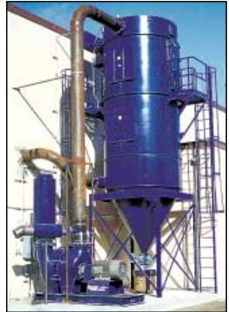
Power Mizer vacuum producer with pulse-type separator providing a continuous duty, high velocity dust collection system at a printed circuit board manufacturer.
